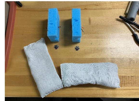
Figure 6: Completed cotton covers coupled with two (2) haptic motors and two blue sponges.
