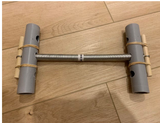
Figure 2: 300 mm spring with hooks, and two plastic pipes measuring 6 ½ inches in height that act as handles.
